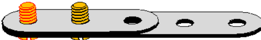
Figure 2. Another Perforated Strip added to the Bolt.
