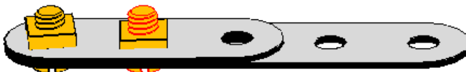
Figure 3. The Nut in the rightmost position is not correctly positioned.
